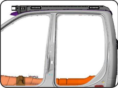
Align and center the rack into place on the vehicle. Once the placement of the rack is satisfactory, mark the mounting locations onto the masking tape by tracing the tab and the hole. Remove the rack from the vehicle and set aside. Make sure the light bar is installed when marking the hole locations. (Remember: "Measure Twice, Cut Once") Double-check that the rack is centered and that the marks are in the correct location.
