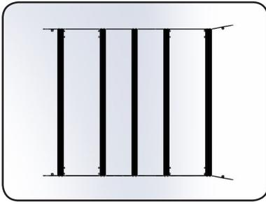
After all the desired carriage bolts have been installed, fasten the remaining side rail to the extruded cross bars, as done so in Step #1. Once attached, ensure all screws are securely fastened. See Step 11 for mounting the LED light bar. Once the light bar is installed and both side rails are attached the rack is fully assembled.
